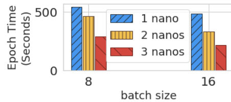
Figure V.4: DL model training time (per epoch) for different resource configurations and different batch sizes.
