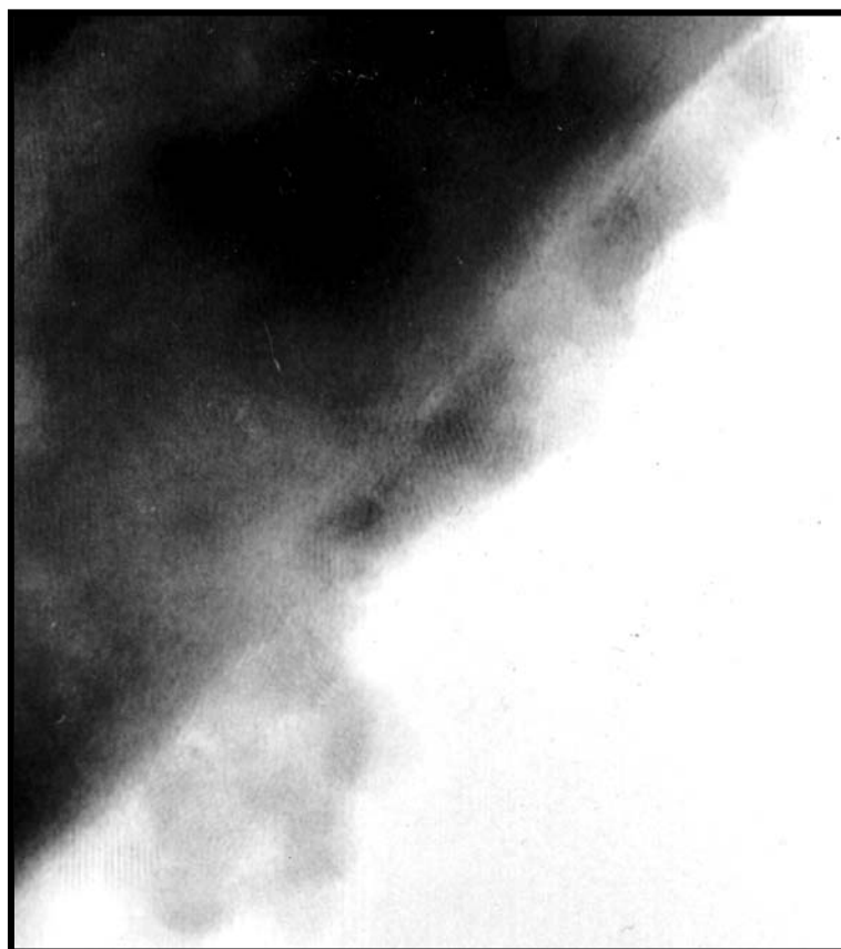
Figure 16. TEM Micrographs of nanocrystals on the surface of TiO 2
