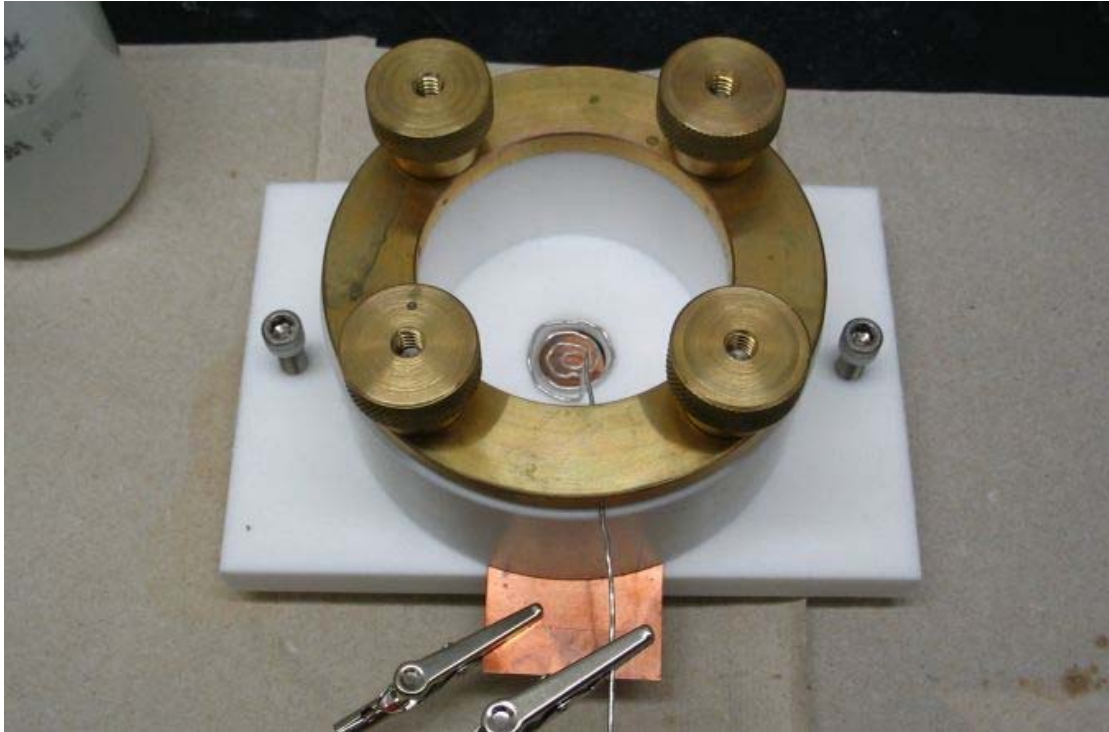
Figure 7. The anodization etch cell
