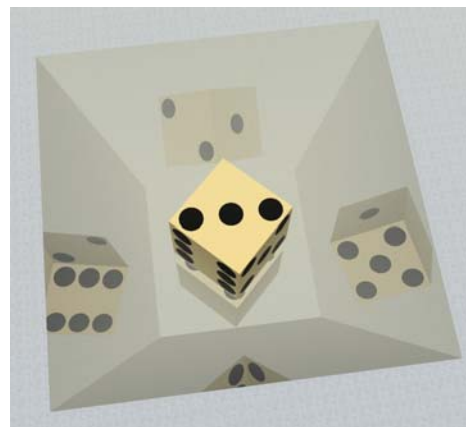
Fig. 1. A dice in a mirrored well. Information about each of the six faces is available.
