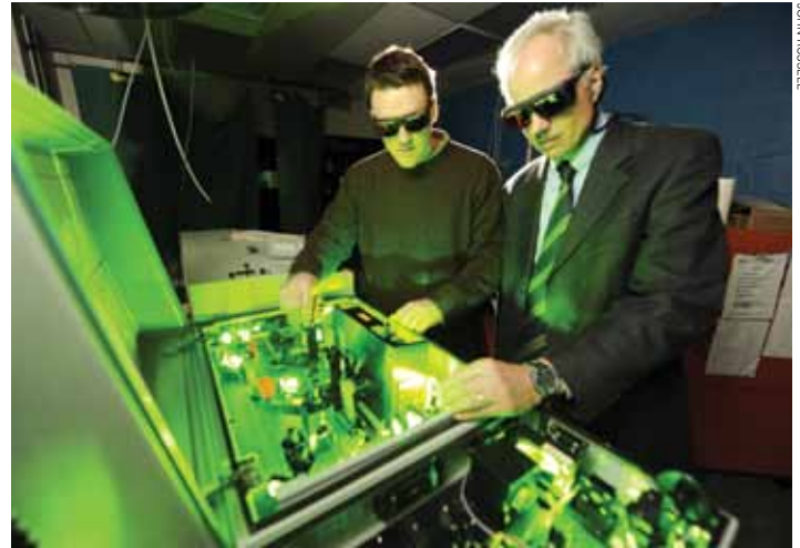
Graduate student Marc Ramsey (left) and Pitz use lasers to split, tag and then measure molecules. The goal is to understand how similar molecules would react at hypersonic speeds.
