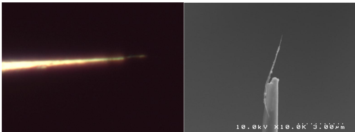
Figure 3 a) Optical microscope image (1000x) of tungsten needle tip and CNT bundle after mounting procedure. b) SEM image of same specimen, showing the bundle attached to the needle, with a single nanotube protruding from the tip.
