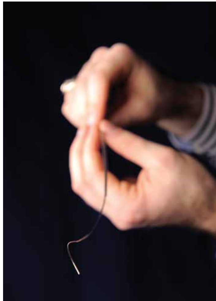
Webster and his team continue to refine steerable surgical needles. This one consists of a series of telescoping precurved tubes that are flexible and can rotate inside each other.
