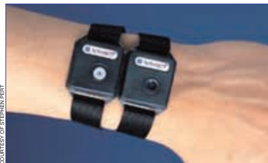
An actigraph, or movement sensor, measures movement and helps researchers track sleeping and waking patterns without doing sleep studies.
