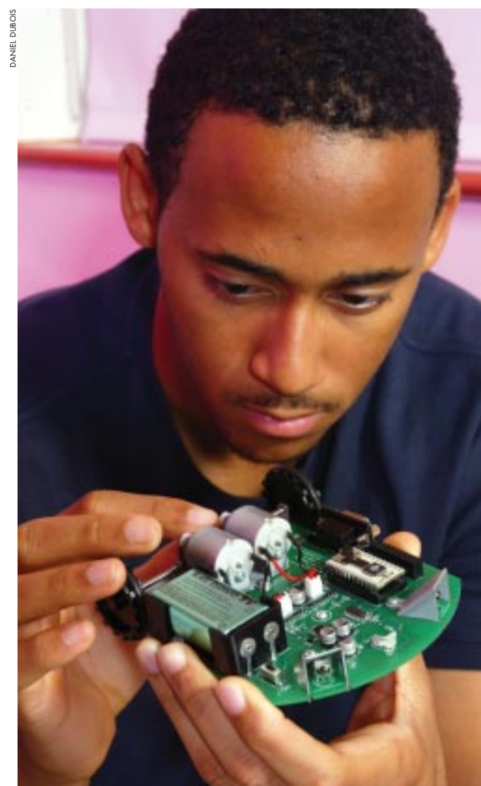
Michael Rivera-Jackson with the parallax robot he programmed to detect upcoming collisions and avoid them.
