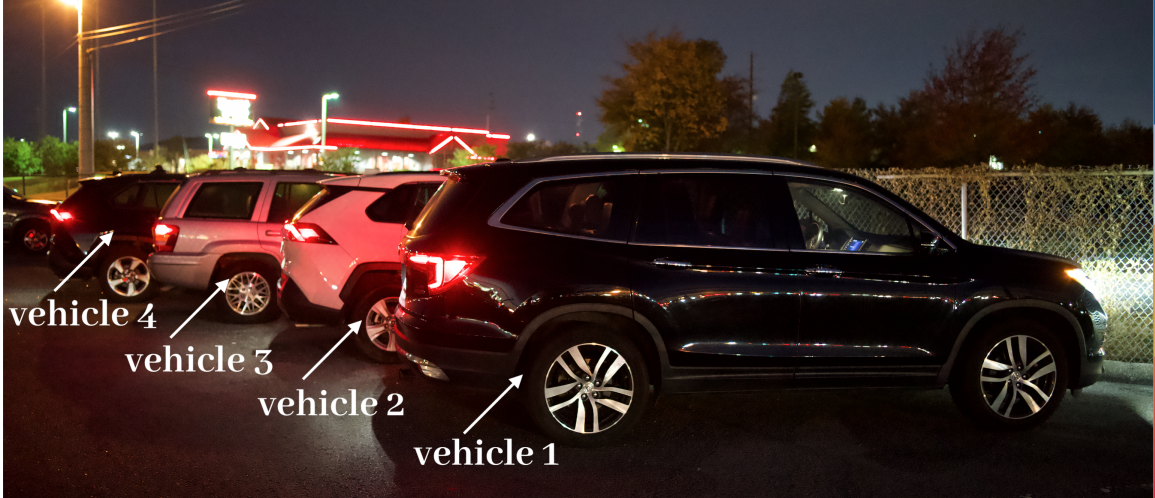
Figure 7.5: Experimental Deployment: Four vehicles, pictured here, are launched into early morning congestion on Interstate-24. From right to left, they enter into the traffic flow. Vehicles 2 and 4 are instrumented for experimental control, and vehicles 1 and 3 are operated under human-piloted control.
