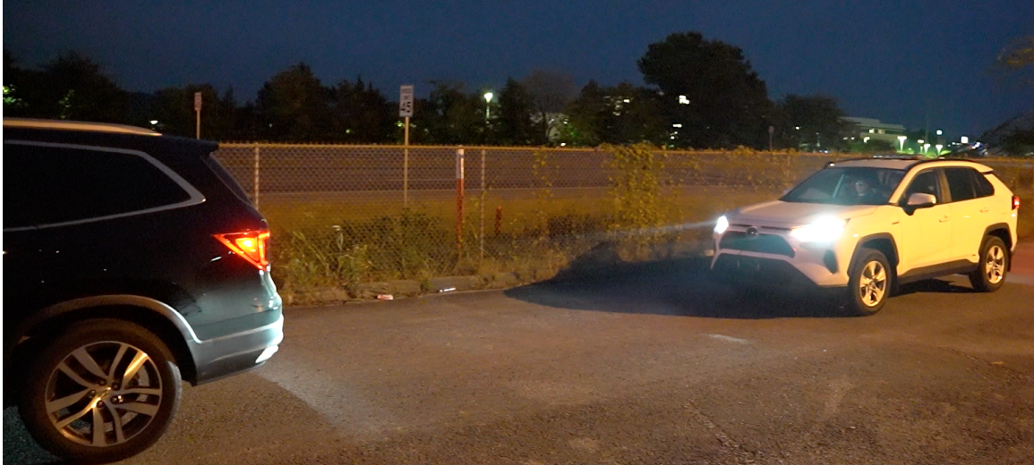
Figure 6.2: Control vehicle (right) preparing to deploy as a VSL-following CAV on I-24 behind pilot vehicle (left) for trajectory comparison.
