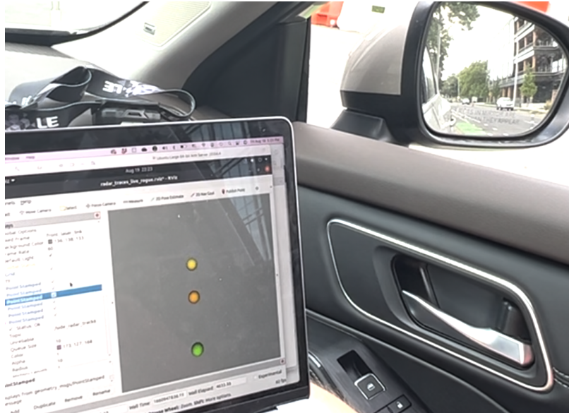
Figure 9.3: In situ CAN decoding is facilitated in ROS, thanks to the ability to project messages from multiple signals into visualization engines that can help in correlation.
