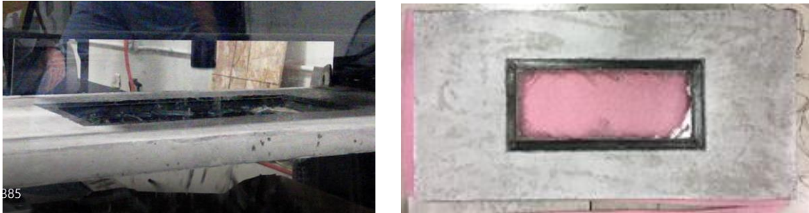
(a) View of test in progress (b) Glass pane blown away, no damage to concrete
