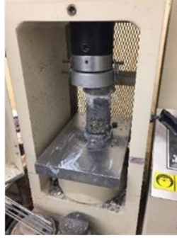
Figure A3. Unconfined compressive strength testing of concrete.
