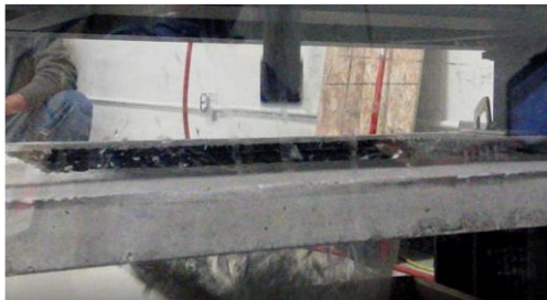
(a) Shattered glass pieces captured by poly-film
