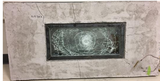
(b) Back face primary crack across the width
