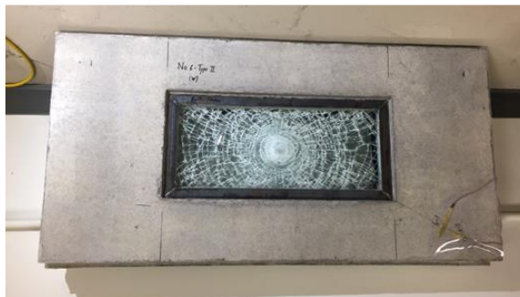
(b) View of back face damage
