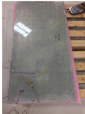
Figure 4.5. Type-I panel after polyethylene film placement.
