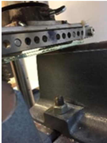
Figure A6. Four-point flexure testing of glass strip using Tinius-Olson UTM.
