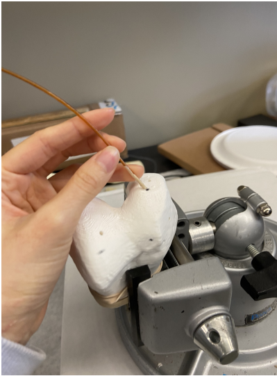
Figure 2.12: Top view of tracing the surface of the knee model with the FOSS fiber sheathed in polyamide tubing
