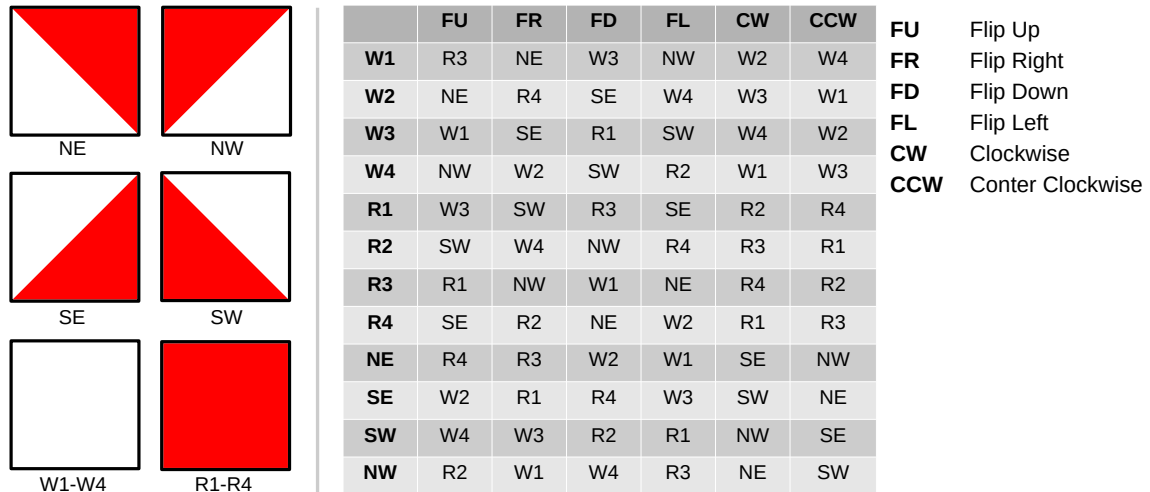
Figure 3.15: The internal representation used to store block states and transitions for the block design task.
