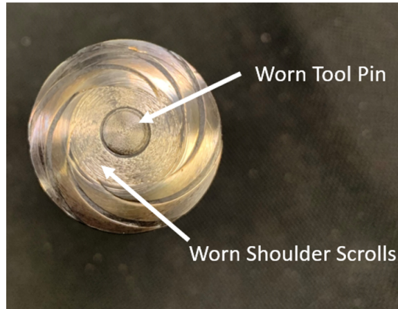
Figure 6.17: Worn tool shoulder and pin from carbon fiber abrasion.
