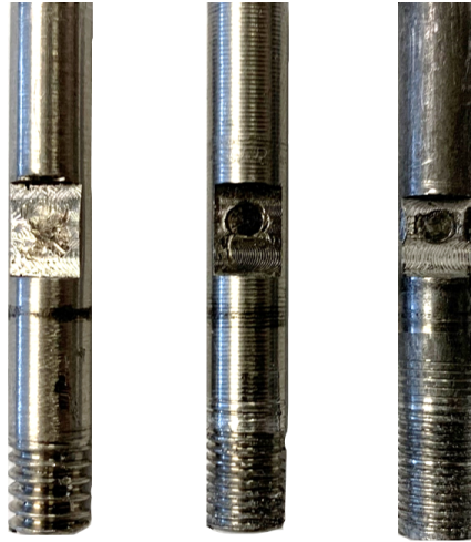
Figure 3.2: Three tool thread pitches used in this study. a) 1.27 mm (20TPI) b) 0.79 mm (32 TPI) c) 0.58 mm (44 TPI).
