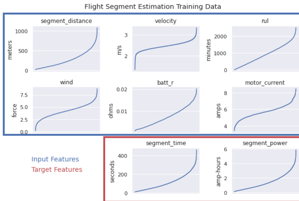
Figure 5.12: Input data plots for the flight time and power estimation model, sorted by value to show range of inputs.
