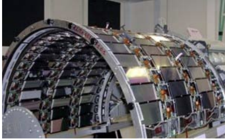
Figure 5.6: Half of the strip detector inner barrel (TIB). [16]
