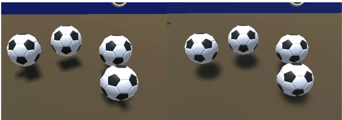
Figure 3.2: Hard shadows (left) vs soft shadows (right) on a virtual desk.
