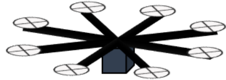
(b) Octo-rotor UAV manoeuvres by controlling propeller speeds.
