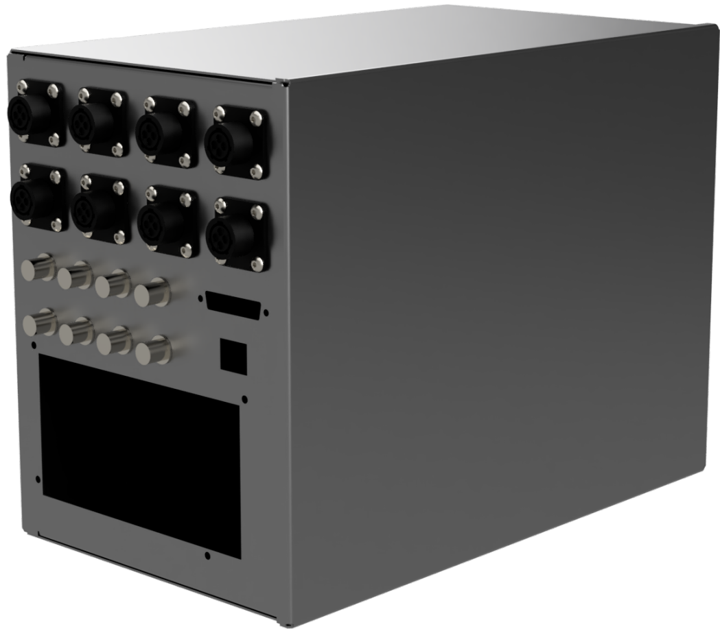
Figure A.3: Render of the case constructed to hold the power supply and signal conditioning for the positional feedback system.
