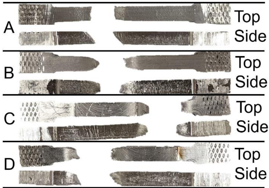
Figure 42. Select specimen fracture behavior with top and side views. A: Base material. B: Base material with heat treatment. C: FSW joint in ambient conditions. D: FSW joint with heat treatment.
