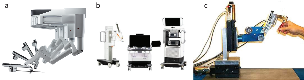
Figure 1.4: Figure of examples of robotics in surgery: a) Intuitive daVinci Xi for laparoscopic abdominal procedures [9], b) Medtronic Hugo for laparoscopic procedures [10], c) JHU steady-hand for precision alignment and tremor accommodation in microsurgery [11].
