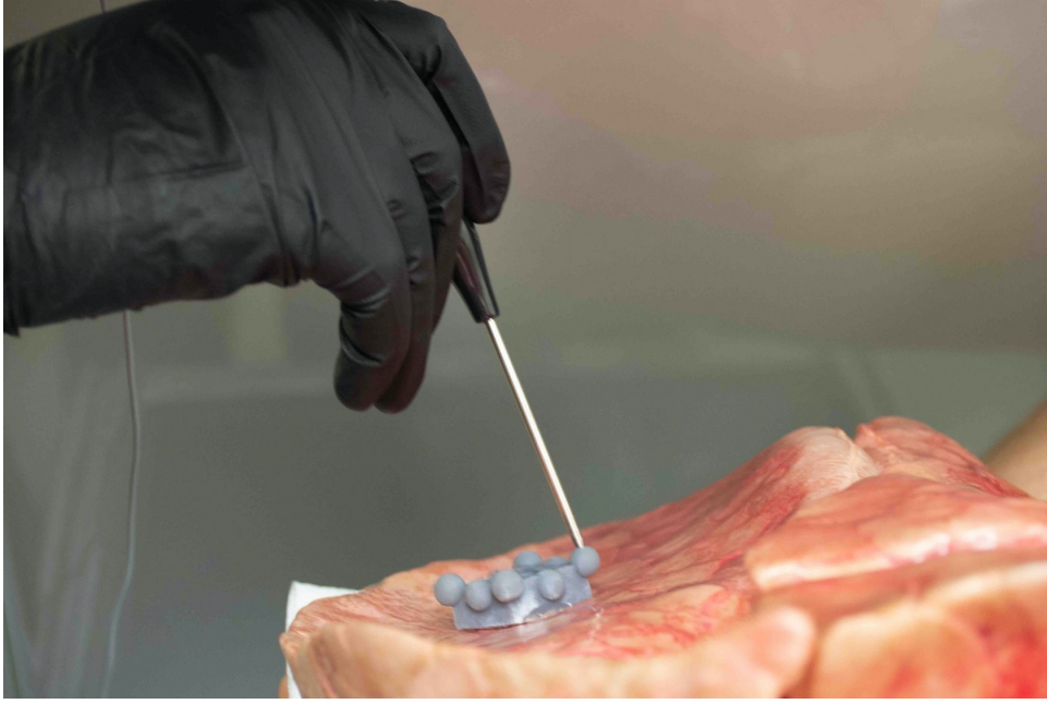
Figure 2.10: Each of the points of the plastic markers is required for rigid registration of the EM tracker to the CT frame. Initially, this was performed by probing the points with a 6DOF EM tracked probe; future versions leveraged 6DOF live-tracked markers that were precalibrated using this process to enable faster registration in the workflow, as described in Equation 2.3
