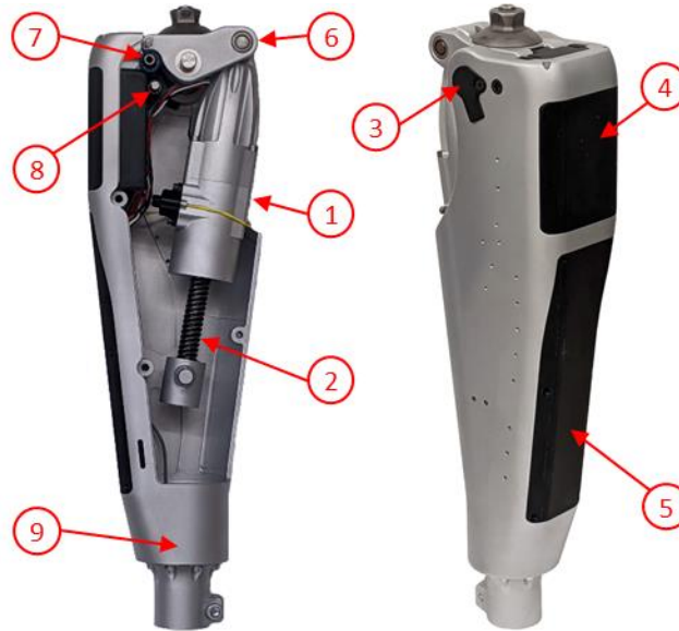
Fig. II-8: ECT knee prosthesis prototype with one half of the housing removed (left) displaying the novel actuator (1) and lead screw (2), and fully-assembled prosthesis (right) including absolute encoder (3), battery pack (4), and custom embedded system (5). The range of motion of the crank arm (6) is limited by the hard stops for extension (7) and flexion (8). The load cell (9) is fixed to the bottom of the prosthesis and attaches to the pylon clamp.
