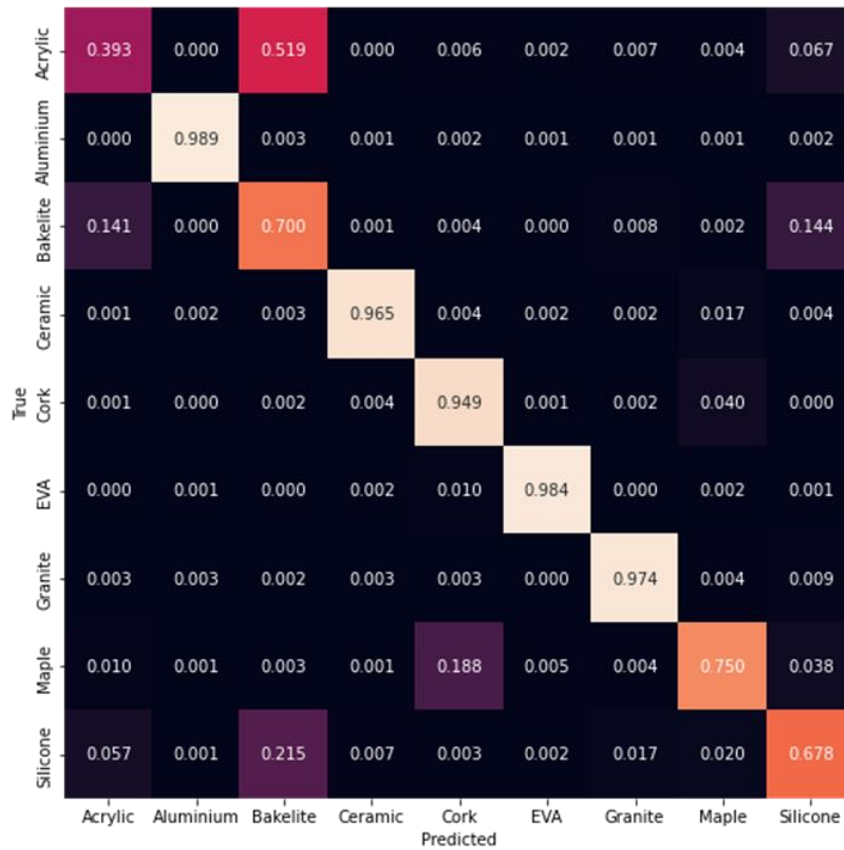
Figure 15: A confusion matrix of the predictions given by M-SMFFNet across all temperatures in the test set.
