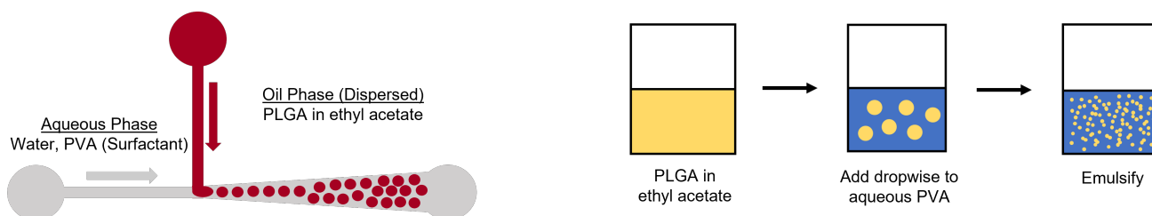
Figure 11: The two methods being compared against to determine if microfluidic-assisted fabrication (left) improves monodispersity of resulting particles compared to the benchtop bulk emulsion (right)
