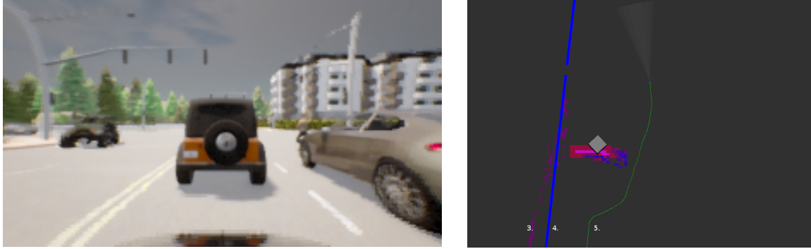
Figure 6.4: Screenshots from each autonomous system simulation. The left figure shows an image from the forward-looking camera of the AV as it navigates through the city. The right figure shows a top-down view of the UUV where the vehicle (trajectory shown as a green line) is inspecting a pipeline (thick blue line) until an obstacle (grey box) is detected by the forward-looking sonar and the vehicle performs an avoidance maneuver.
