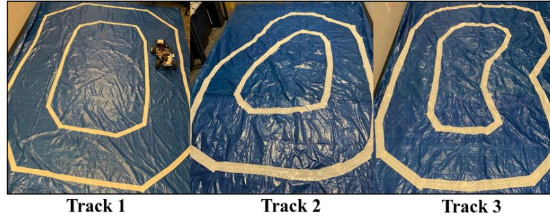
Figure 7.4: We collected data from tracks 1 and 2 to train the LEC and perform exploration for the RL-based decision logic of the dynamic-weighted simplex strategy. Track 3 was used to test the performance and accuracy of the trained LEC and the dynamic-weighted simplex strategy. The tracks were built indoors in our laboratory using 10' x 12' blue tarps. The videos of DeepNNCar performing on these tracks can be found in https://github.com/scope-lab-vu/deep-nn-car
