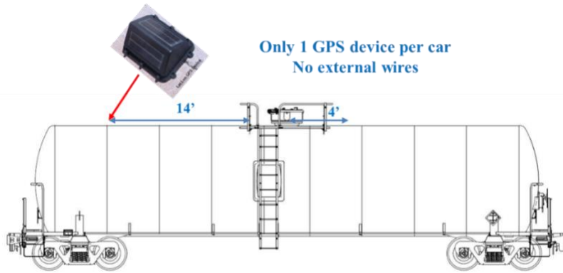
Figure 2.3: Tank Car Equipped GPS Device
