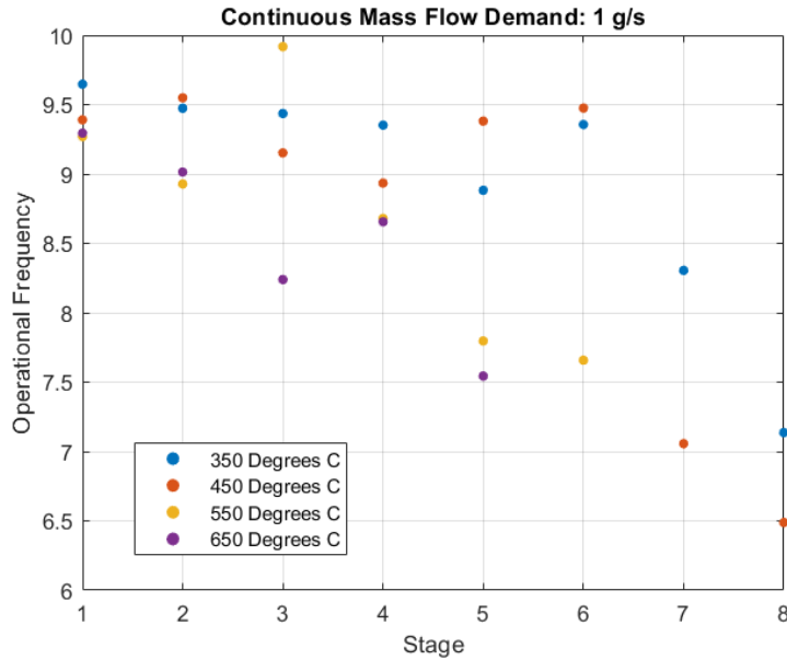
Fig. IV.25: Operational frequency of each stage of multi-stage thermocompressor arrangements for a selected mass-flow demand.
