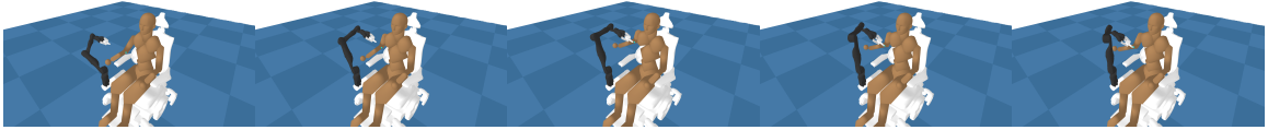
Figure 2.2: Example of our robot completing the itching task even when the human is dis-functionally moving its arm upward
