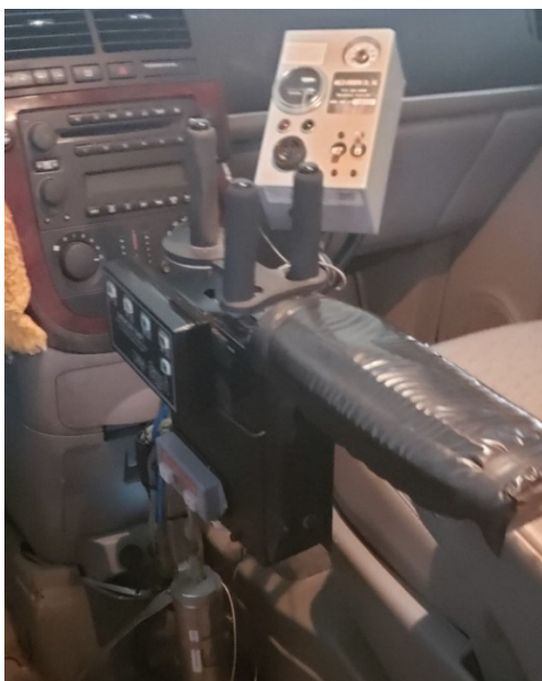
Figure 4. Hand Controls and Armrest for Vehicle
