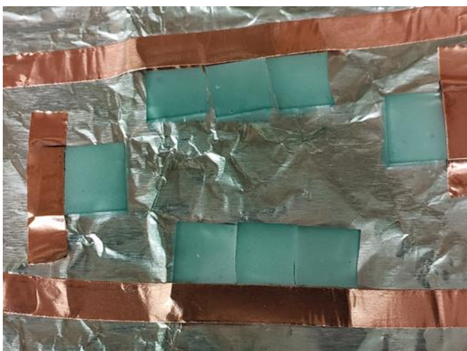
Figure 5.8 Anodes with electrospun PANI/CSA fibers directly onto the TiO_2 np layer.
