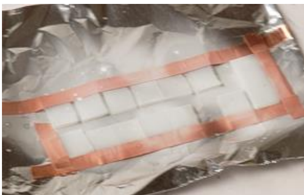
Figure 5.7 SEM of \text{TiO}_2 nanoparticle layer showing vertical three dimensional structure. Image of anodes after electrospay \text{TiO}_2 nanoparticles, prior to sintering.
