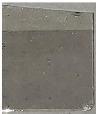
Figure 5.4 ITO anode with sputtered 30nm \text{TiO}_x Blocking layer
