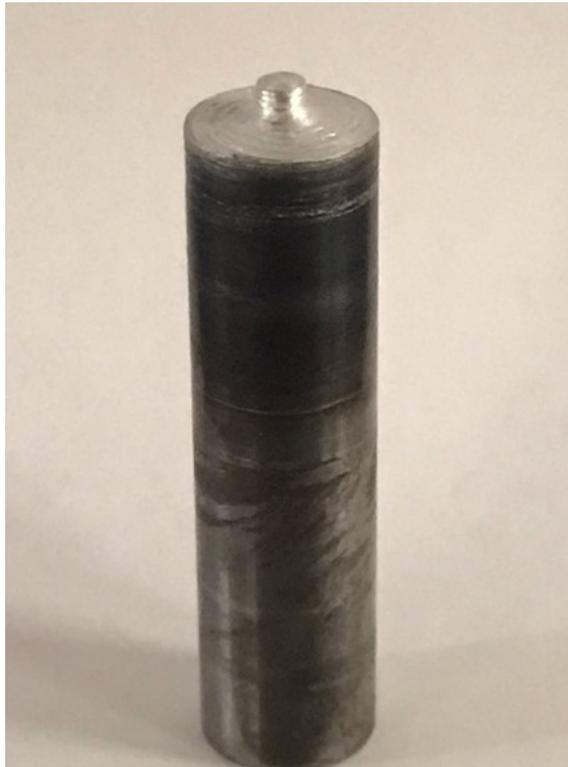
Figure 3.4: FSW tool selected for this thesis, featuring a scrolled shoulder and threaded pin. There is some aluminum embedded in the threads and scrolls, but this does not impair function as under operating conditions any material on the tool surface is plasticized.
