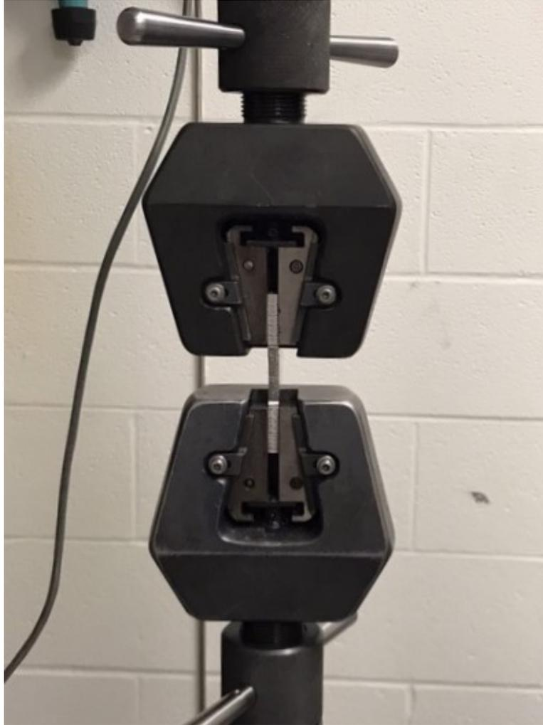
Figure 4.2: Instron tensile tester used for determining sample strength properties.
