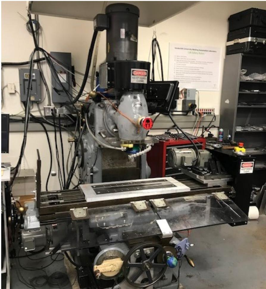
Figure 3.3: VUWAL converted Milwaukee Model K manual mill FSW welding machine.
