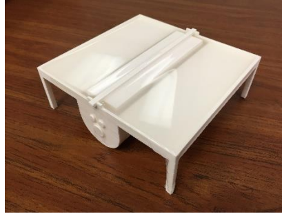
Fig. 18. Silicone wrap curing in 3D-printed mold
