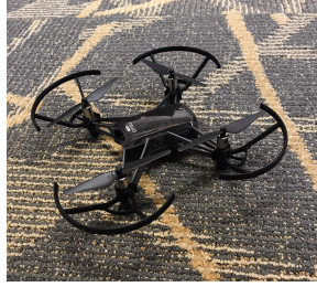
Figure III.4: The DJI Tello Edu quadcopter drone used by the students in the course.
