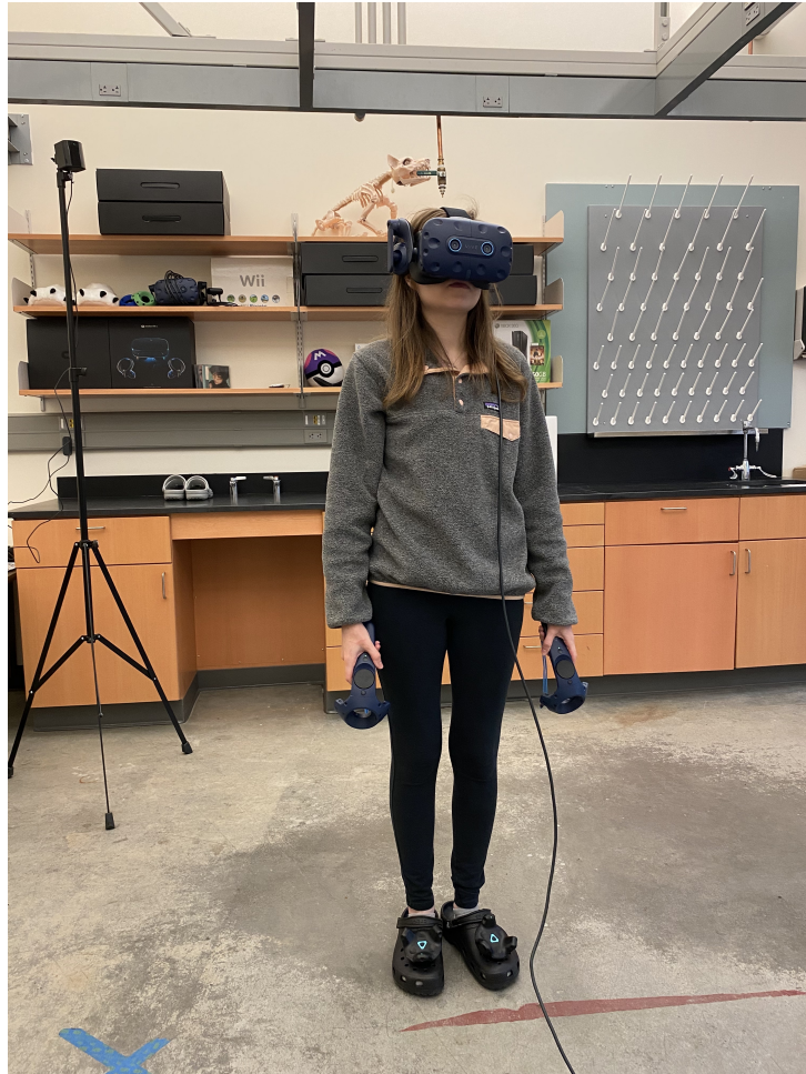
Figure 16: The equipment used in both experiments. As seen, the Vive Pro HMD was worn, along with the handheld controllers and two Vive Trackers placed on the feet.
