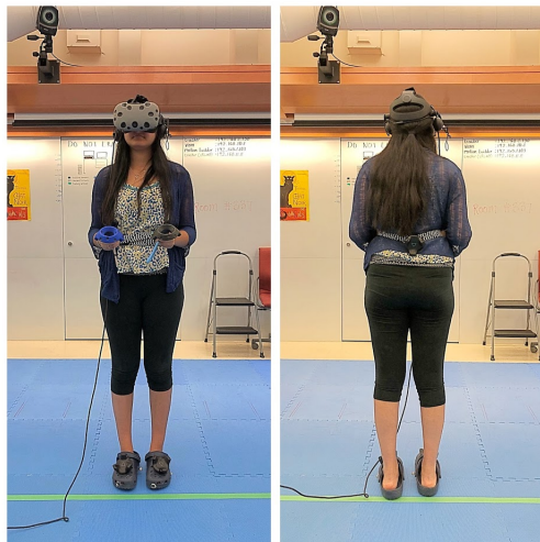
Figure 8: The equipment participants used in both Experiments 1 and 2. Along with the head-mounted display and handheld controllers, Vive trackers were attached to both feet and the middle of the lower back via shoes and a belt. ©IEEE 2020
