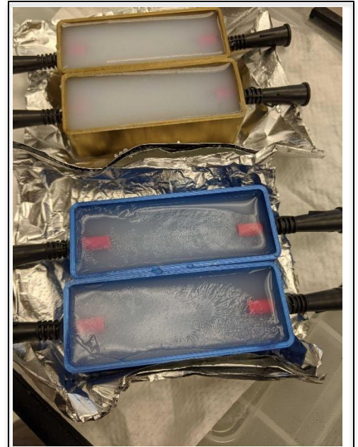
Figure 6. Artificial silicone vessel cannulated on both ends with 10 Fr female urinary catheter, sealed with heat shrink tubing, and mounted within a 3D printed box. The enclosure was then filled with PVA cryogel solution and subjected to four freeze-thaw cycles to form the gel. The top two phantoms pictured are 10% PVA cryogels, while the bottom two phantoms shown are 6% PVA cryogels.
