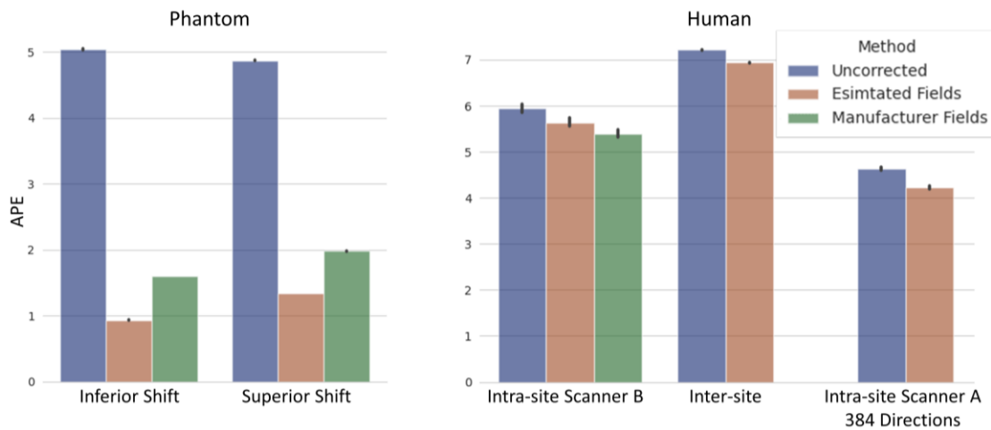
Figure IV-9. The mean APE within the phantom and brain excluding CSF regions are shown for each experiment without correction, after correction with the estimated fieldmaps, and after correction with the manufacturer specifications when available.
