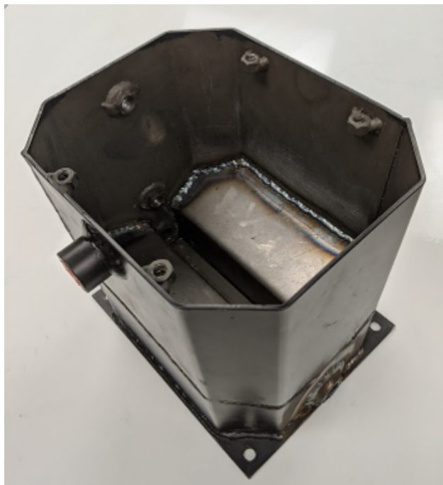
Figure 2.6 Benchtop facility reservoir with internal modification.
