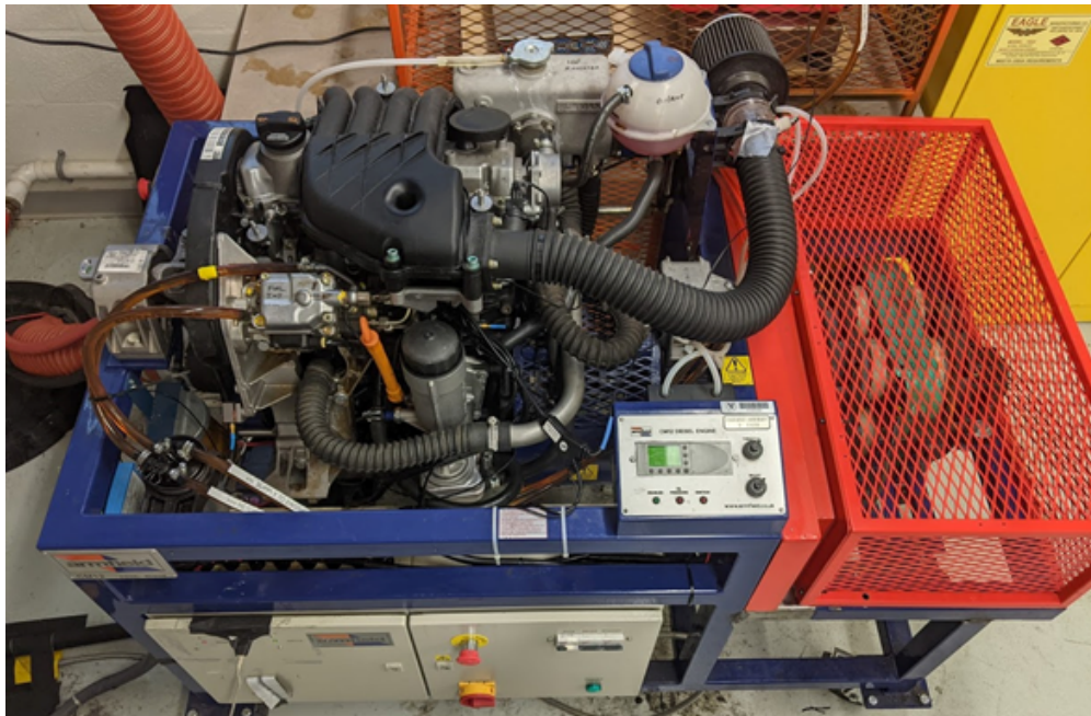
Figure 1.2 Testbed Volkswagen 4-cylinder, 1.9L TDI diesel engine with dynamometer.
