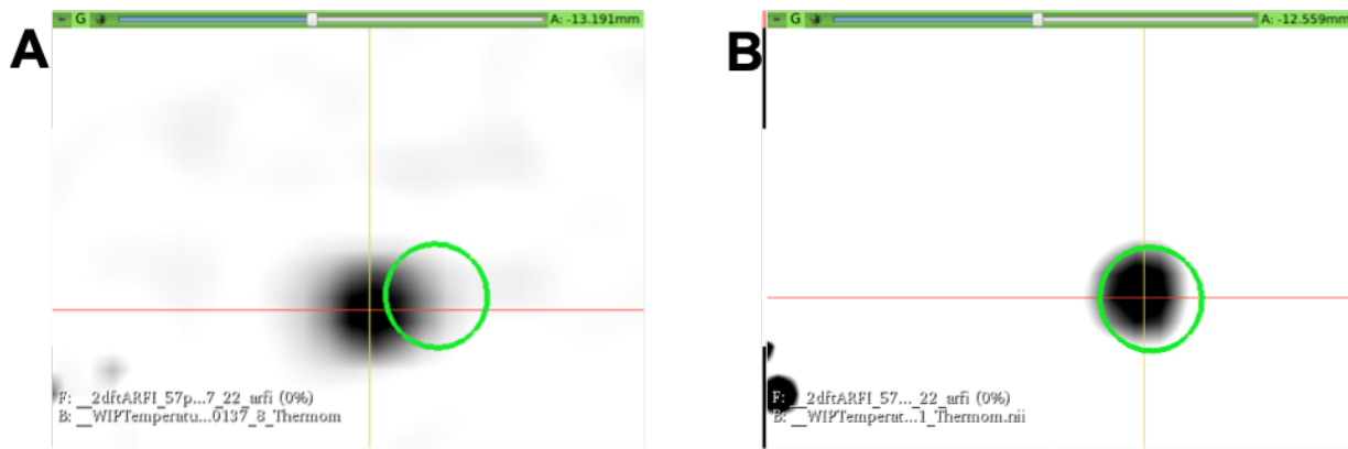
Figure 5.5: An example of the lateral bias in the initial tracker to ultrasound transformation. A: The optically predicted focus is shown with the green circle and MR thermometry shows a focus location that is laterally shifted from this focus. B: Even without bias correction we are able to use the thermometry derived location of the focus to steer the beam to the optically predicted location.
