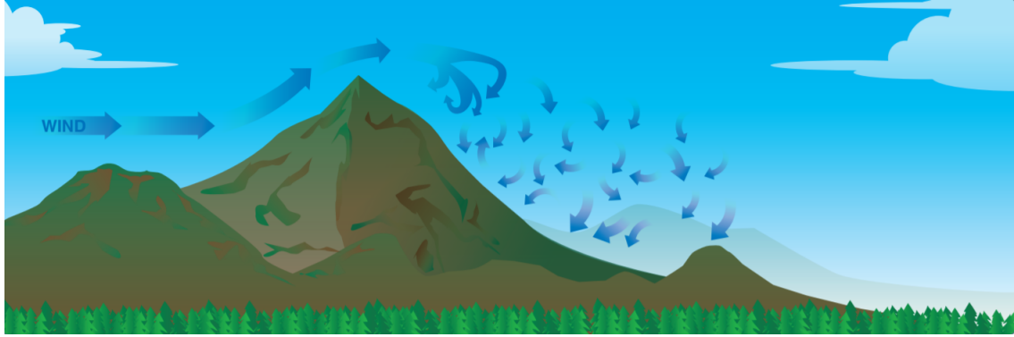
Figure 3.1: Turbulence generated by wind passing over surface obstructions. The planetary boundary layer by definition lies above such turbulence.
