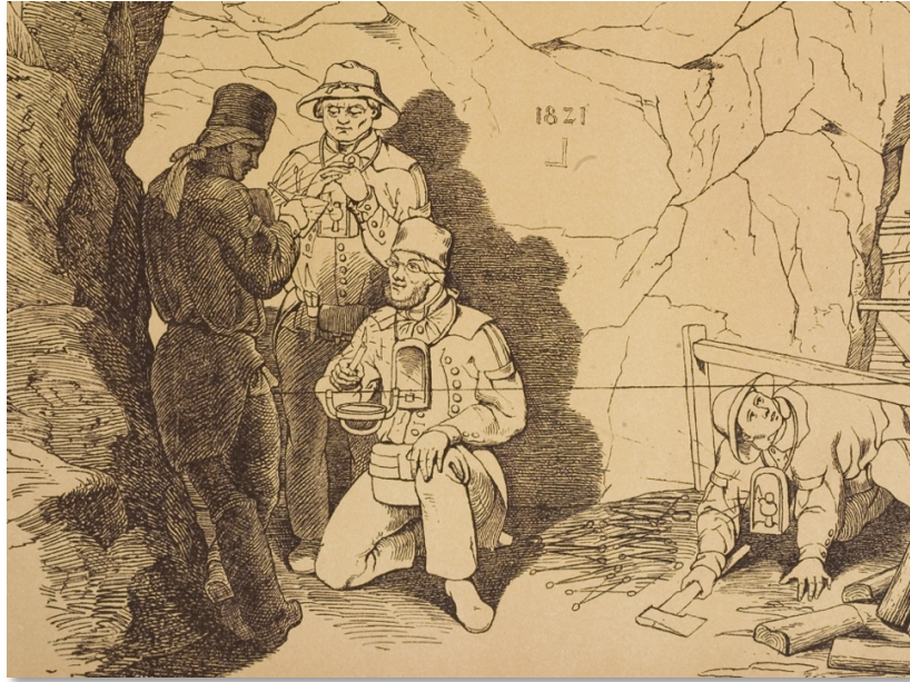
Figure 3. Surveyors at work measuring the mines, recording degrees from the Hängecompass . Eduard Heuchler, Die Bergknappen in ihren Berufs- und Familienleben bildlich dargestellt und von erläuternden Worten begleitet (Dresden: Kuntze, 1857), Plate 17, with description on p. 7. The author-illustrator was himself a professor at the Mining Academy. Max Planck Institute for the History of Science, Library, Rara H592b.
