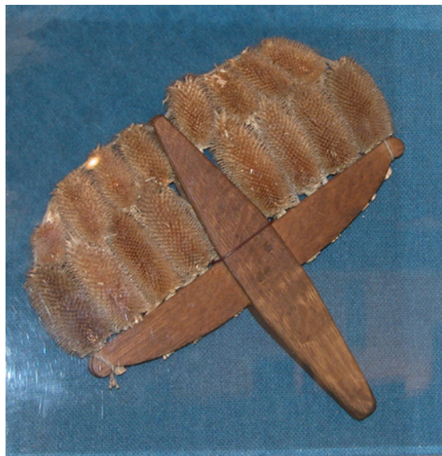
Figure 3. Traditional teasel cross for carding wool, at the “Clothworker’s Exhibition” in Lavenham, Suffolk in 2005. © National Trust Collections, Photo: Sue James, CMS_LAV317_14.
