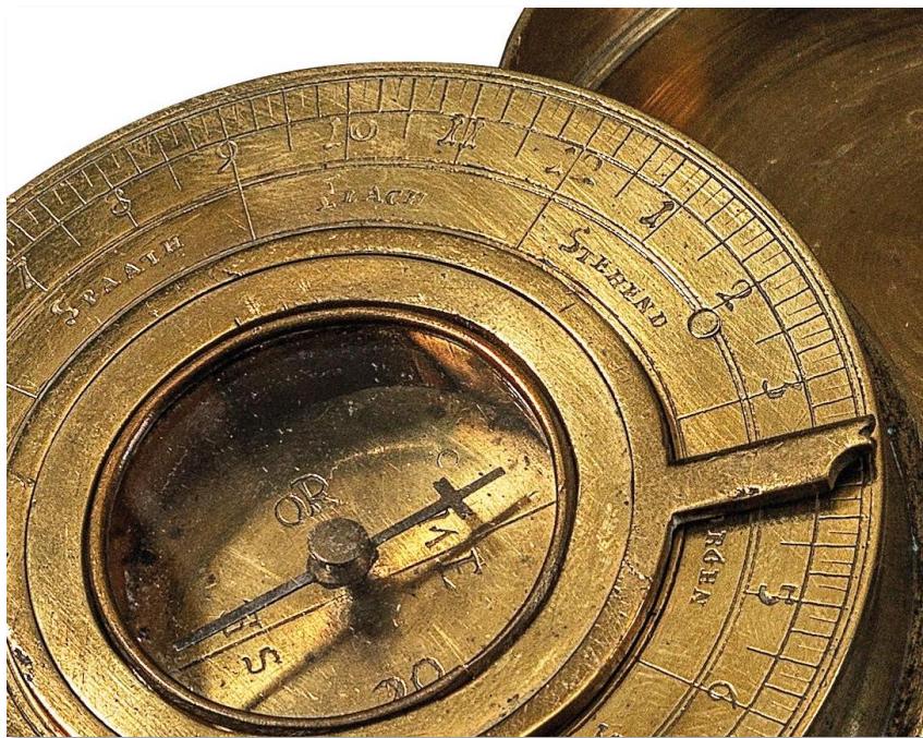
Figure 4. A brass Bergcompasse , 72 mm in diameter, of seventeenth- or eighteenth-century origin. The declination Spaath corresponds to OR , striking eastward as Humboldt instructed pupils, while Stehend aligns with the tail of the magnetic needle pointing to ME , or meridies . This means “Mittag,” the word used in eighteenth-century Germany to designate south (where the sun stands at mid-day). Photo credit: Dorotheum Vienna, auction catalogue 25.09.2019, Lot Nr. 336.
