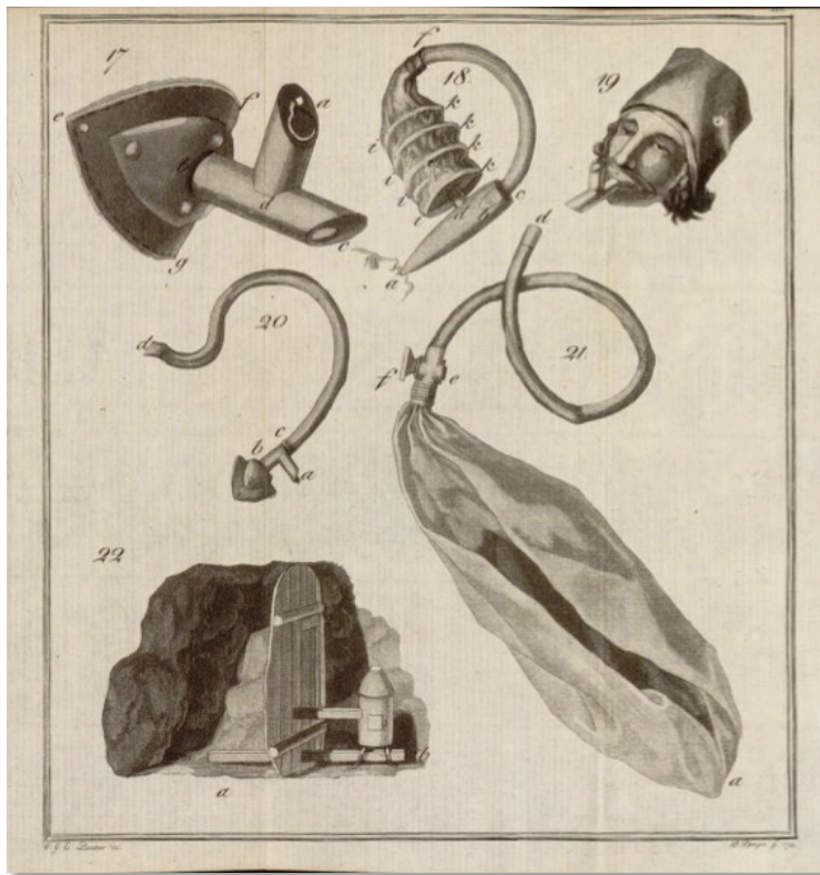
Figure 1. Humboldt's self-made respiration device, or Rettungsmaschine , for miners caught in böse Wetter , as illustrated in Ueber die unterirdischen Gasarten (1799). SUB Gö, 8 Metall 2933.
