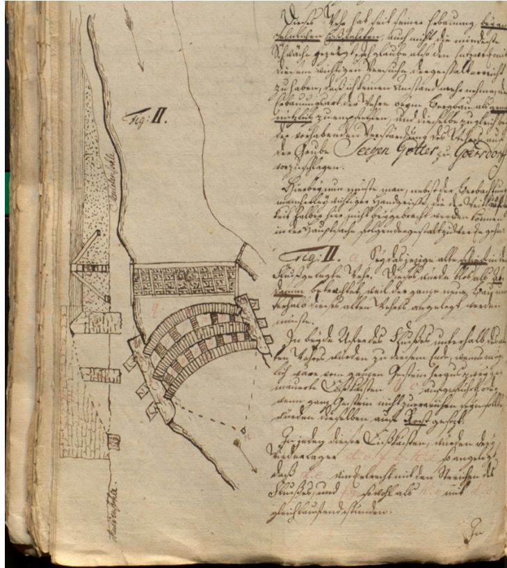
Figure 5. The “fortress” on the Mulde. In Mende’s sketch, we see both the original wooden weir and the three stone arches of its proposed replacement. The sluice that opens to the canal is shown just above the wooden weir, to the right. SächsBergAFG 40174, Grubenakten Freiberg 643, Bl. 81.
