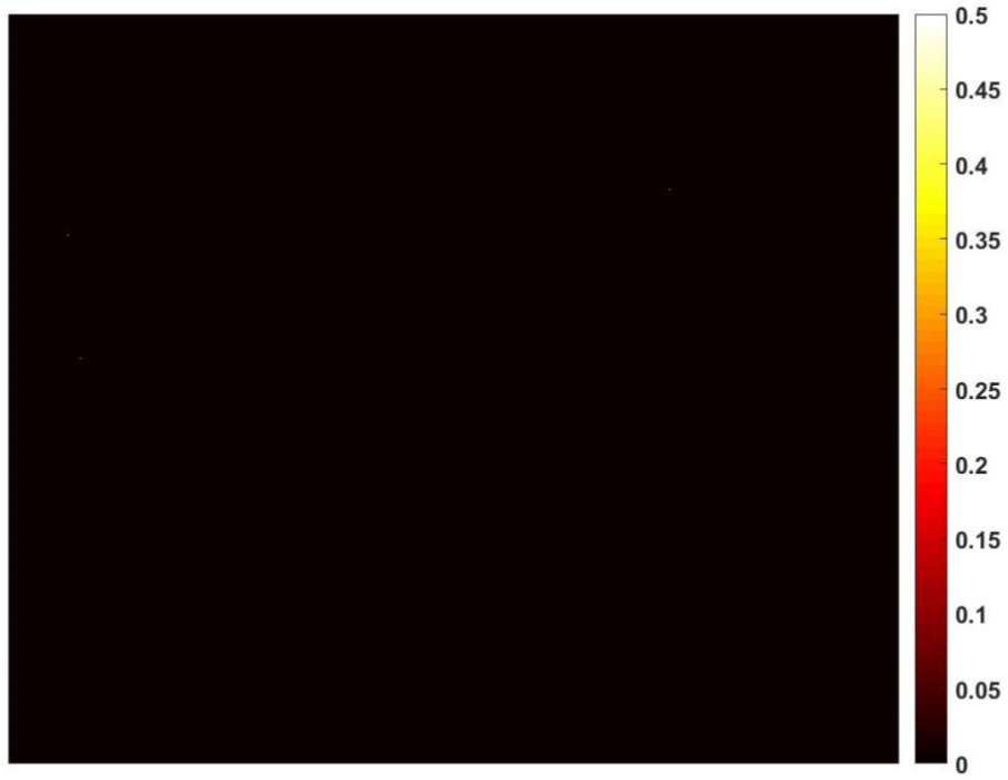
Figure 51: Centroid image of the non-gated background measurement imaged in alpha mode with 13 total detected counts.
