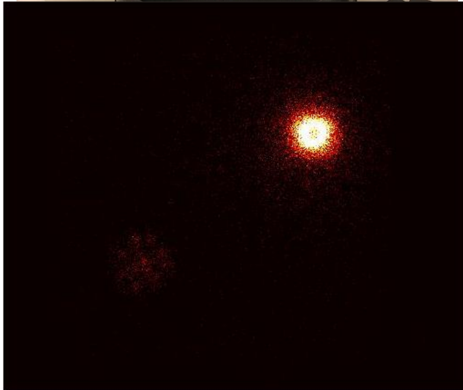
Figure 68: (Top) Example setup of beta/gamma discrimination measurements of LA iQID imaging. ^{241}\text{Am} (red button source) with tungsten collimator (flat round disk of metal under the red button) and ^{99}\text{Tc} (silver one with white sticker). (Bottom) Actual sources used for particle discrimination MATLAB algorithm, ^{241}\text{Am} in top right and ^{90}\text{Sr}/^{90}\text{Y} in bottom left.
