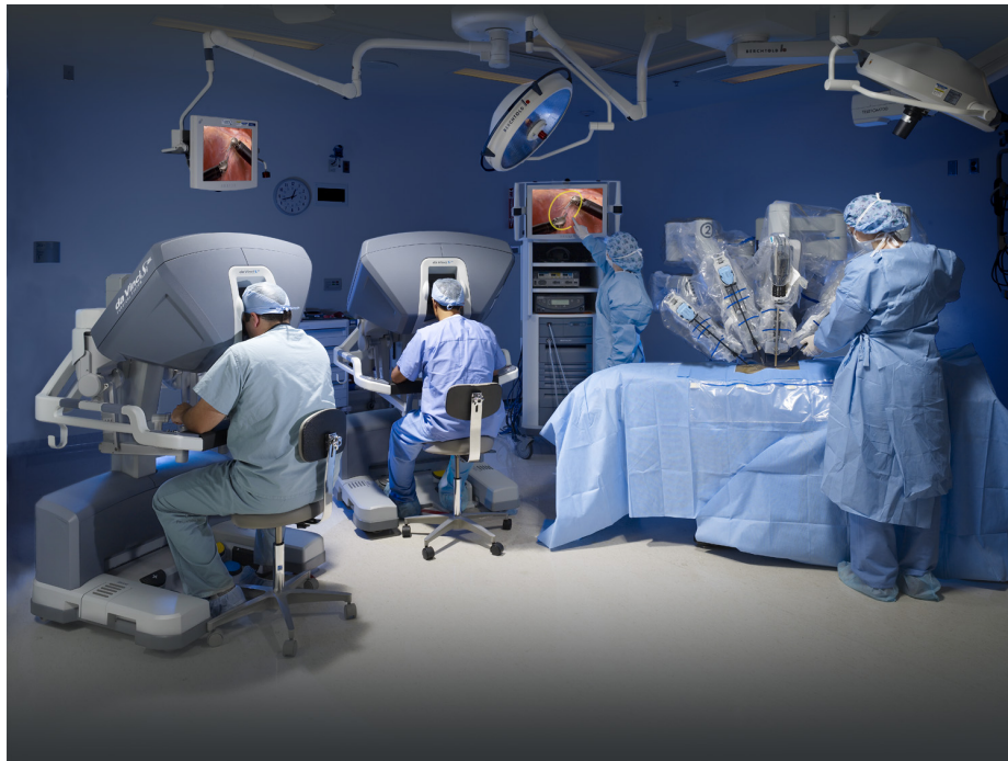
Figure 1.1: The da Vinci Xi surgical robot is operated remotely by a surgeon sitting at a console.
