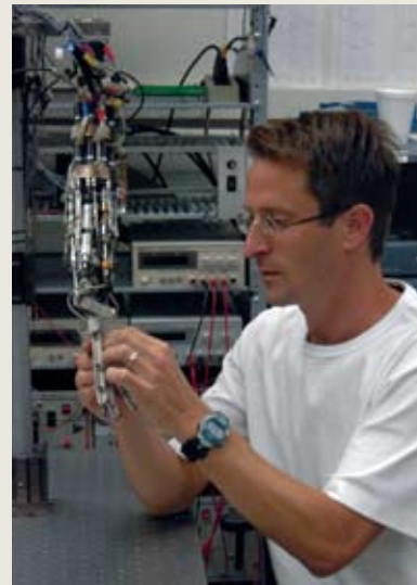
FRANCIS SIMPSON / The Vanderbilt Hustler The robotic arm, powered by hydrogen peroxide, is a state-of-the-art prosthesis that will provide an alternative to current prostheses in the near future. Michael Goldfarb led the project with the intent of creating a robotic arm prosthesis that will eventually integrate into the human body.
