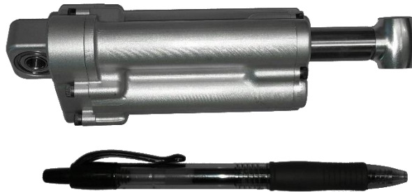
Fig. 2.4: Photograph of constructed PAL actuator and pen (for scale).
