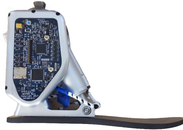
Fig. 3.3: Constructed prototype of the semi-powered transtibial prosthesis with visible embedded system.
