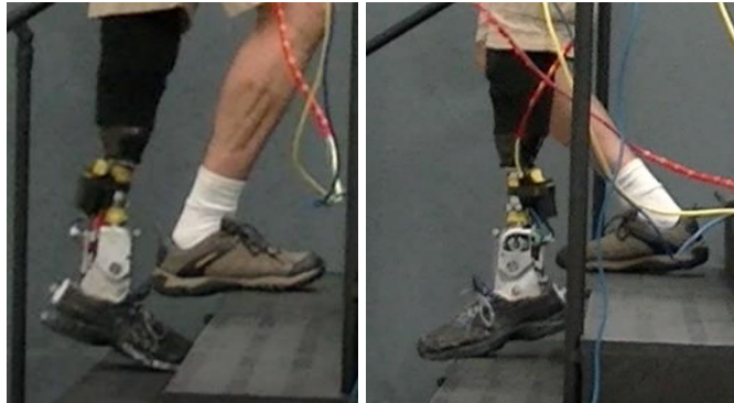
Fig. 5. Vanderbilt transtibial prosthesis prototype during stair ascent and descent, including integrated battery pack, and also showing CAN cable for supervisory control and data acquisition.
