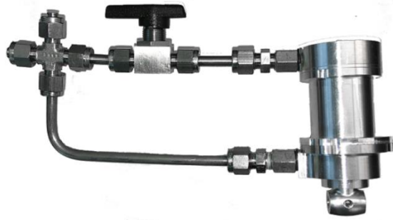
Fig. 4.5. CVHA shown in closed test circuit with ball valve in between cylinder ports. The capped connected shown was used for filling, but sealed off during the experimental characterization.
