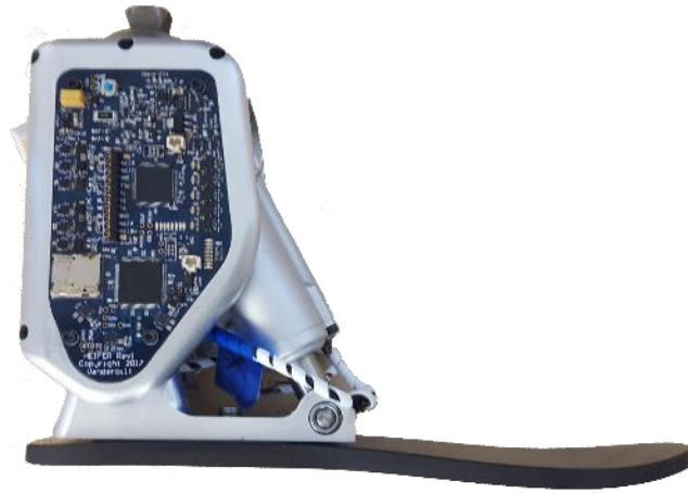
Fig. 2.6. Photograph of the constructed ankle prosthesis. The ankle embedded system can be seen on the side of the device (blue). The battery is housed in the posterior portion of the device and not clearly visible in the figure.
