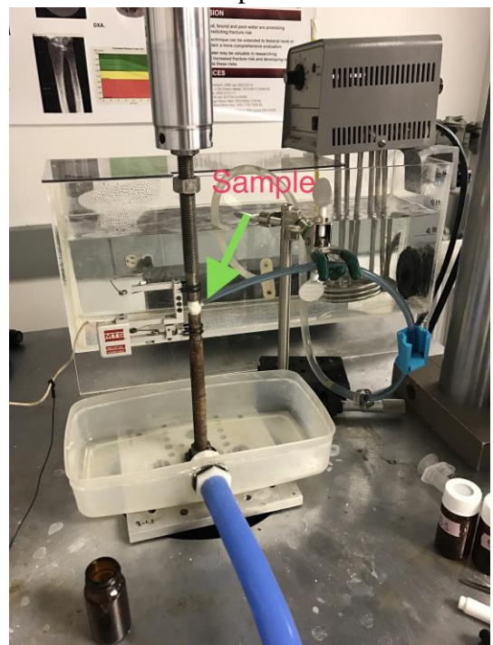
Figure A1. MTS setup for fatigue testing.
