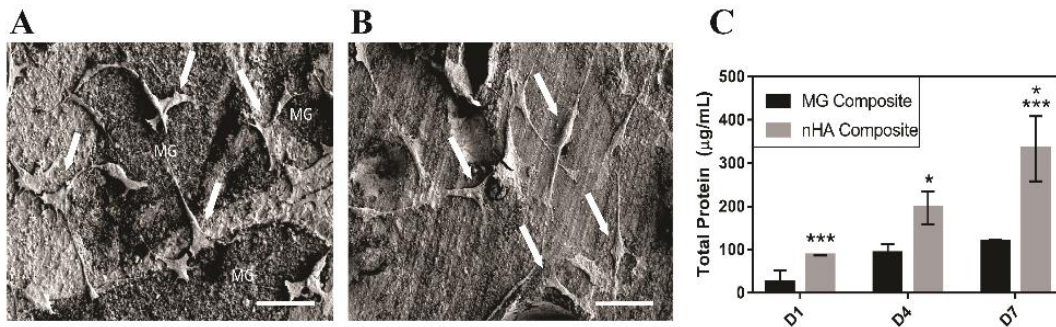
Figure 3.6. MC3T3 cells (arrows) attached and spread on (A) MG and (B) nHA composites after 24 h incubation. Scale bar = 50 µm. (C) Measurements of total protein versus time indicate that cells proliferated faster on nHA composites.
