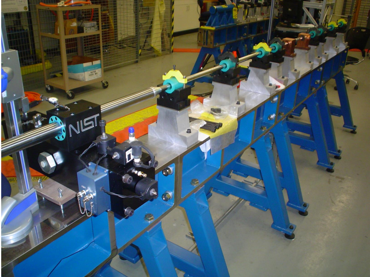
Figure 3-10: Kolsky-Bar setup at the National Institute of Standards and Technology in Gaithersburg, MD.
