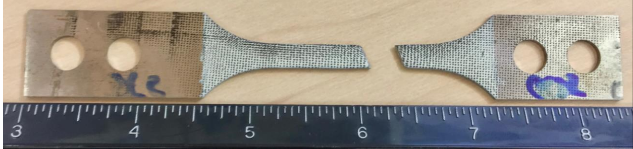
Figure 3-8: Tensile specimen pulled to failure at \dot{\epsilon} = 10^1 /s (note the pin-loading holes). The image is used to show the size scale (ruler in inches) of the digital image correlation marks (black ink marks on a white background).
