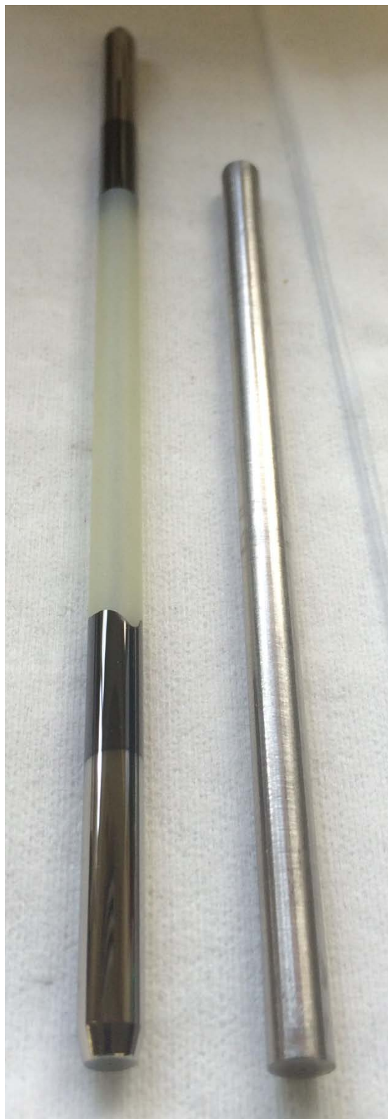
Figure B.19.3: Resistive glass capillary, held up to light and compared to home-built capillary
