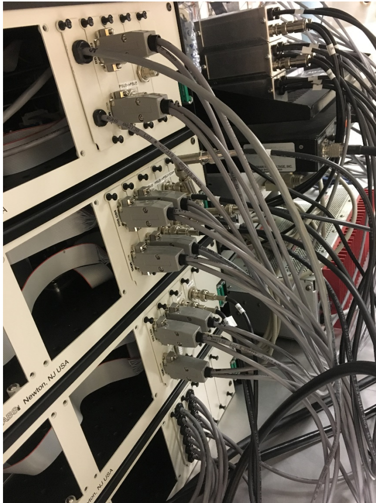
Figure B.19.20: Organization of cables leading from PSUs in drawers to 24 VDC supply, breakout boxes, and NI connector block which connects to NI chassis
