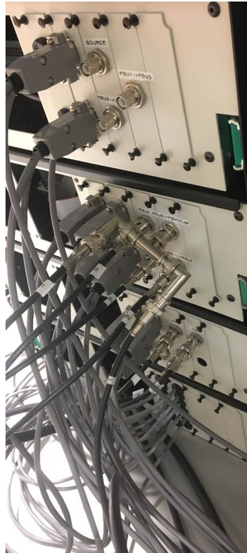
Figure B.19.20: Organization of cables leading from PSUs in drawers to 24 VDC supply, breakout boxes, and NI connector block which connects to NI chassis
