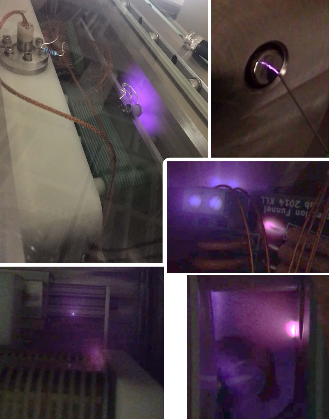
Figure B.19.25: (Counterclockwise from top left) Corona and/or discharge in chamber at aperture panel, drift tube, bottom tab of low pressure funnel, RC circuit board, and outside vacuum between ESI source and RGC
