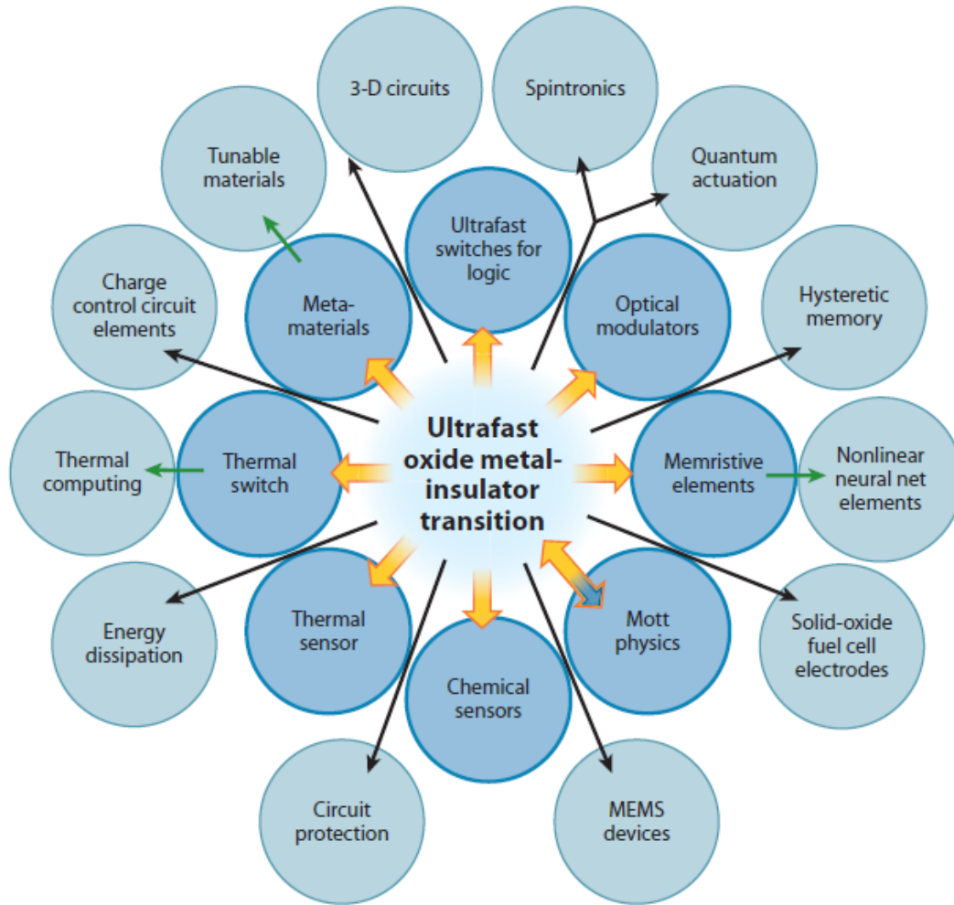
Figure 1.13: Technologies Utilizing IMT in Strongly Correlated Oxides. Device technologies benefitting from the metal-to-insulator transition of strongly correlated oxide. From reference 108 .
