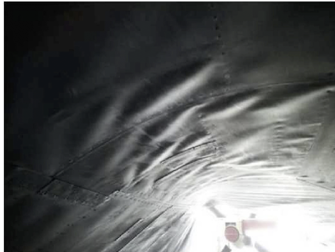
Figure 1.1: Deformation of the Skin Panels on a YF-12 at Wright-Patterson AFB 1 [6]
