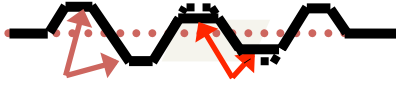
Fig. V-10: Illustration of bit error. An error occurs if the measured voltage level does not reach a percentage of the expected voltage level. This percentage is considered the error threshold.
