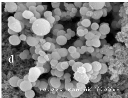
Figure 68: SEM micrographs and histograms of silica nanoparticles produced from the G3 PPI template in concentrations of phosphate buffer of a) 0.5 mM, b) 5 mM, c) 10 mM, d) 20 mM, e) 40 mM, f) 60 mM, g) 80 mM and h) 100 mM.
